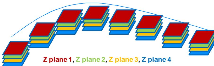
**Figure 7 – Z planes track curved surface**
